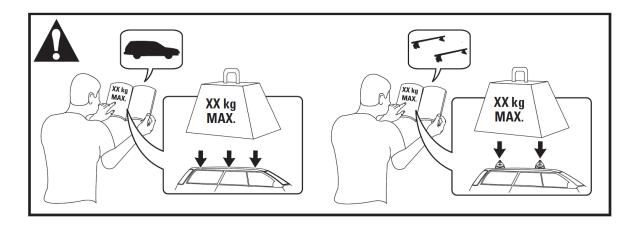
Each of the items listed above has an independent maximum load rating. The maximum amount you can carry on top of your vehicle is the lowest maximum value of all of the components.
